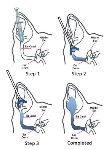
Step 1 shows the application of OticArmor® with a disposable 1 cc syringe, needle removed.
